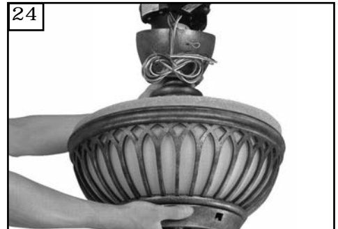
24 Raise fan with downrod assembled to the ceiling bracket and hang fan assembly. Be sure to rotate the downrod ball so that the notch in the bracket engages the slot in the ball.
